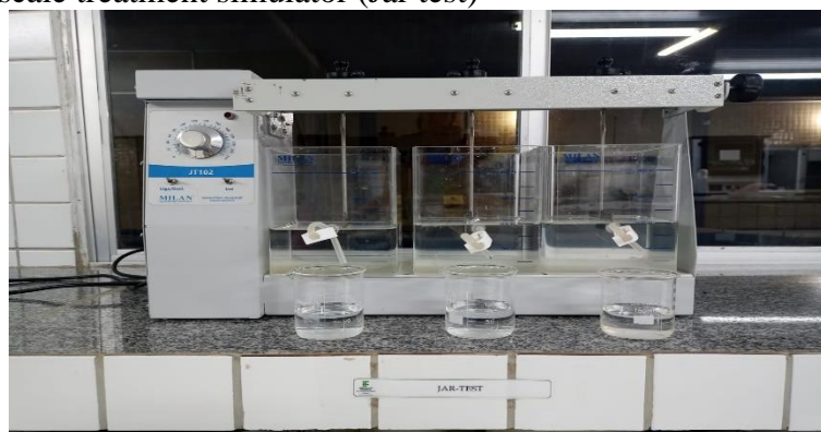
Figure 1. Small-scale treatment simulator (Jar test)
