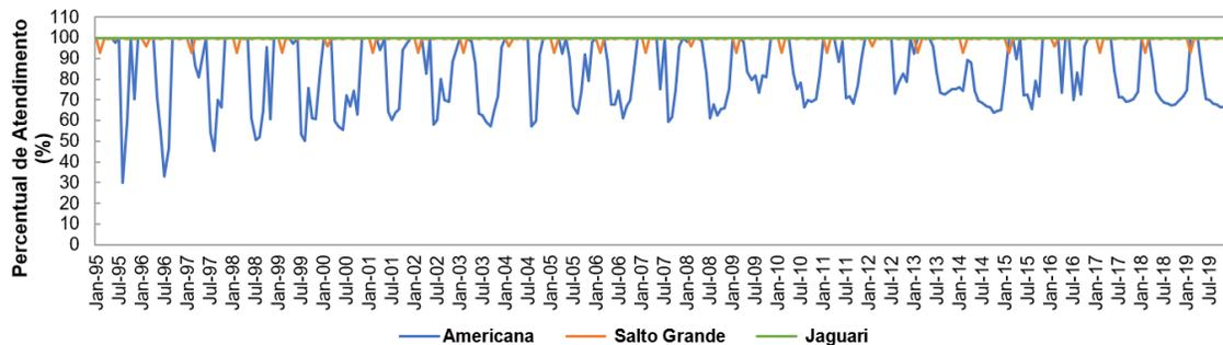
For the Salto Grande and Jaguari hydroelectric plants, the service percentages varied, with Salto Grande maintaining 100% and Jaguari maintaining 93.2% and 100% (Figure 5), reflecting the differences in the turbine flows required to meet their capacities: 34.9  $\text{m}^3/\text{s}$  for Jaguari and 21.5  $\text{m}^3/\text{s}$  for Salto Grande.
