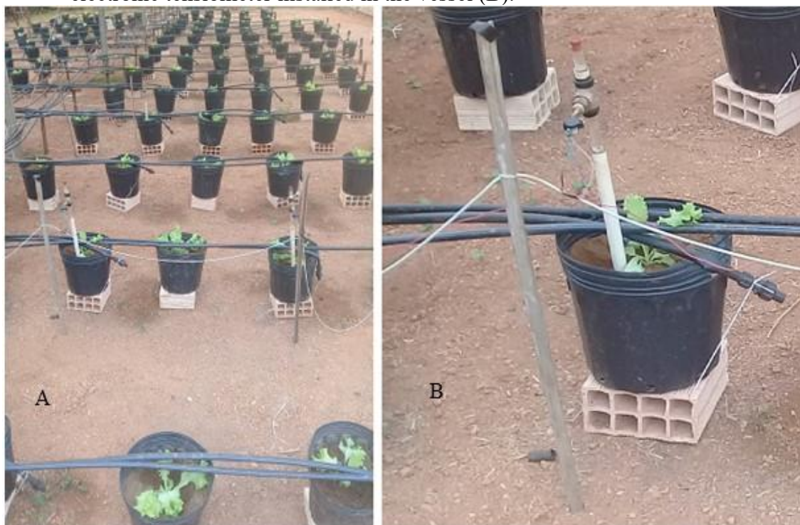
Figure 1. General arrangement of vessels and electronic tensiometers (A); detail of the electronic tensiometer installed in the vessel (B).
