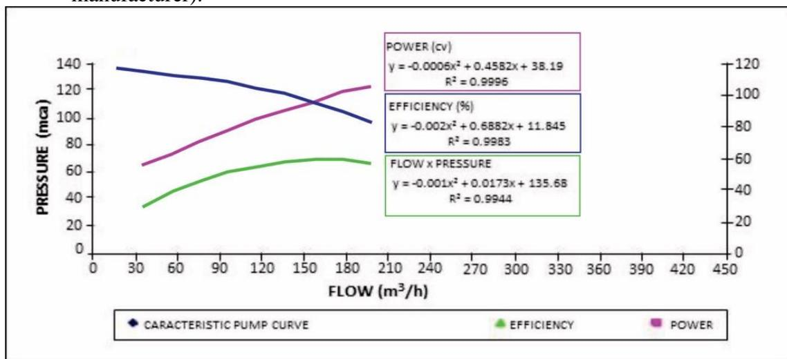
**Figure 5.** Adjustment of the parameter curves of the motor-pump set to parabolic functions with 385 mm rotor diameter and 1800 rpm rotation (best option for the project).
