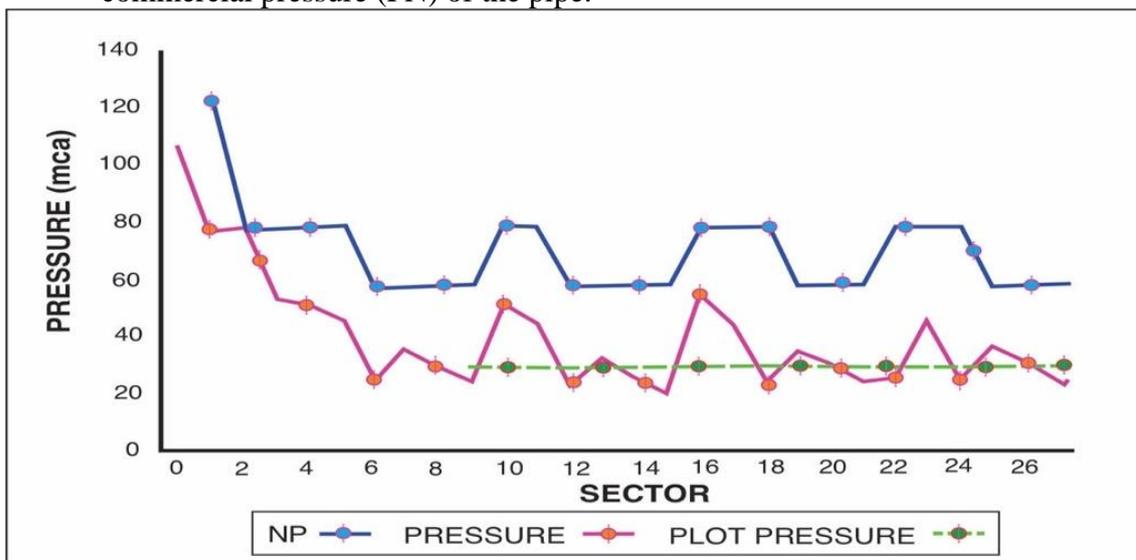
The final design of the pumping system consisted of two diesel motor-pump sets associated in parallel with the following characteristics: pumps with 385 mm impellers at 1800 rpm, a natural diesel engine with six cylinders, continuous power of 67.11 KW, momentum of 32.0 N·m and specific consumption of 162.0 g. (cv·h<sup>-1</sup>) at 1800 rpm. Figure 4 shows the parameters of the motor-pump set for the original pump rotor (405 mm) at its nominal speed (1780
