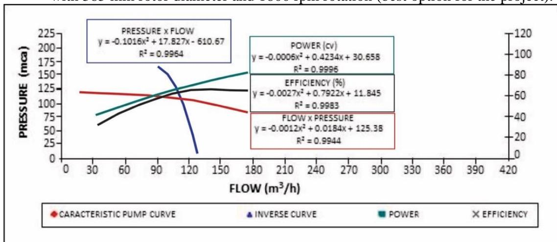
**Figure 6.** Pressure and power curves of the association in parallel with two motor-pump sets, 385 mm rotor diameter and 1800 rpm rotation (final global set).
