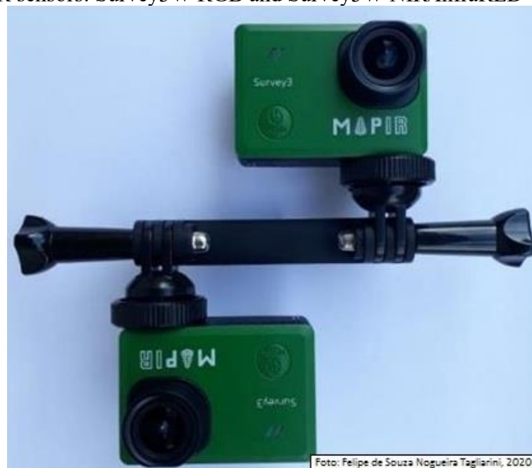
Figure 3. MAPIR sensors: Survey3W RGB and Survey3W NIR/InfraRED
