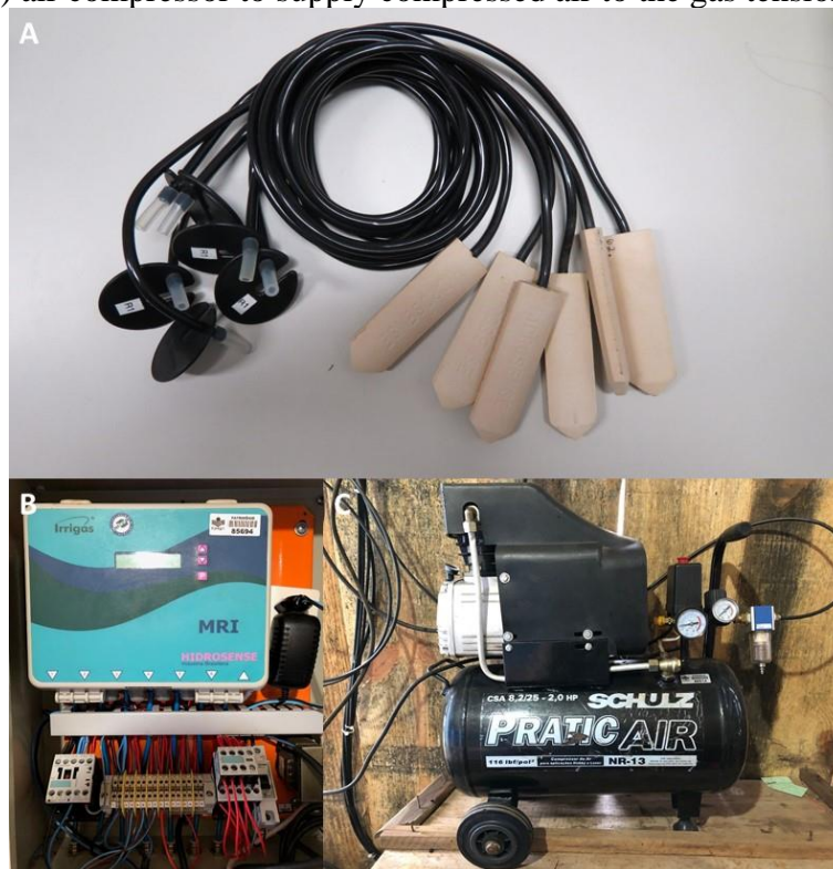
Figure 1. (A) Irrigás® sensors, (B) autonomous irrigation controller based on Irrigás® sensors and (C) air compressor to supply compressed air to the gas tensiometry system.
