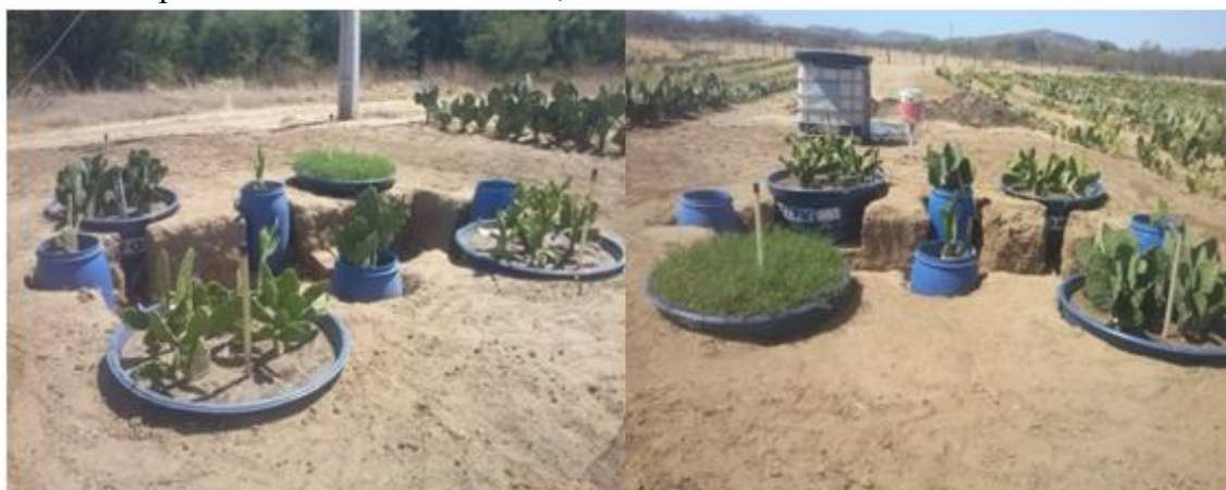
Figure 3. Diagram of the installation of drainage lysimeters for forage palm cultivars in the experimental area. Santa Luzia, PB.
