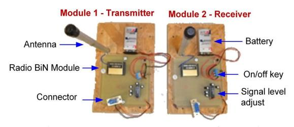
The module radio consumption for the data transmission operation is 17,5mA, which means that a battery type AA (length of 5cm and diameter of 1.45cm) with capacity of 2500mAh could supply this hardware for six days, while a motorcycle battery with 7Ah could provide power for seventeen days. Note that, it is for continuous daily transmission with batteries that can be rechargeable and besides the radio transmitter can also be
