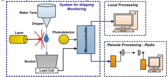
Figure 1. The system for drip emitters monitoring
