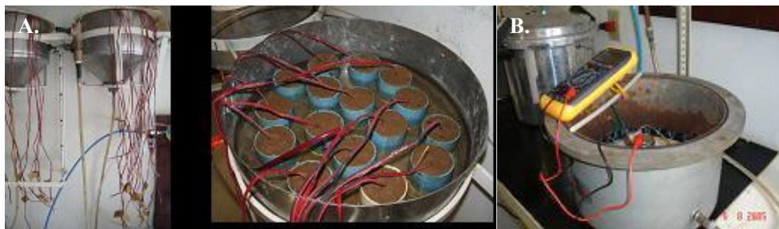
Figure 3. (A) Tension and saturation table of the samples and (B) pressure cooker with soil rings on the porous plate
