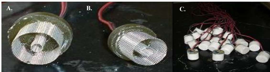
Figure 2. Electrodes constructed with stainless steel screen molds with (A) 20 \times 5 mm, (B) 15 \times 5 mm and (C) encapsulated sensors.
