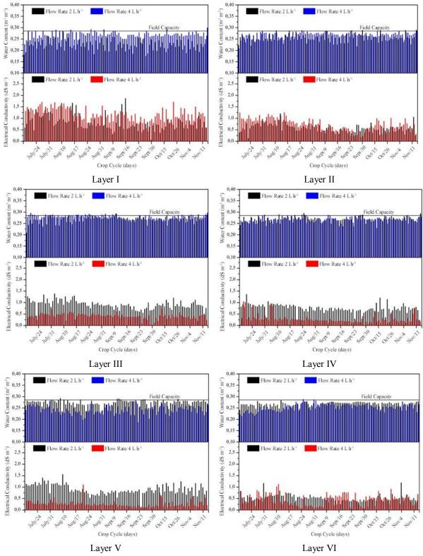
Figure 2. Volumetric soil water content and electrical conductivity of the soil solution in different soil layers for flow rates of 2 and 4 L h<sup>-1</sup>
