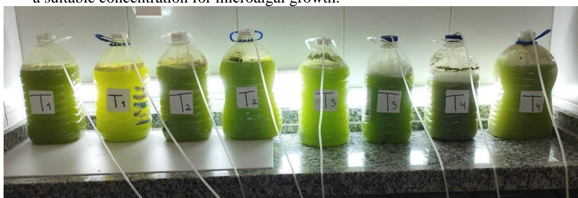
Figure 1. Four whey concentrations, T1: 2%; T2: 4%; T3: 6%; and T4: 8%, were tested to determine a suitable concentration for microalgal growth.
