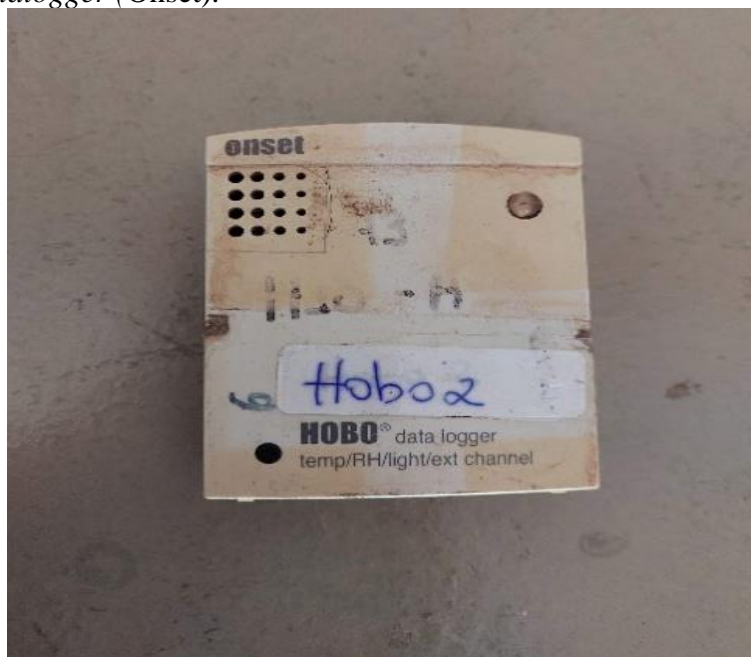
Figure 3. HOBO datalogger (Onset).
