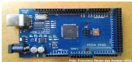
**Figura 3 - Arduino Mega 2560.**
