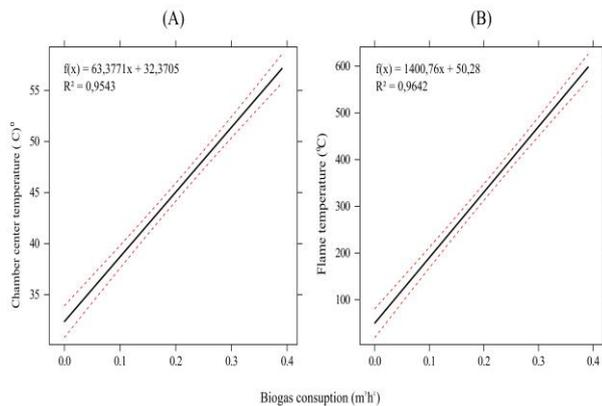
**Figure 2** - Linear regression relating the biogas consumption with temperature in the center of the chamber (A) and in the flame temperature (B)
