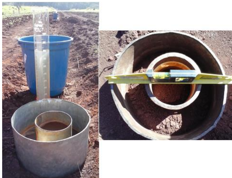
Figure 1. The basic infiltration rate of water in the soil (VIB) was determined via the concentric ring method.
